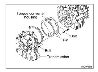
② Using a moving truck slowly, pull out transmission assembly to the front.
