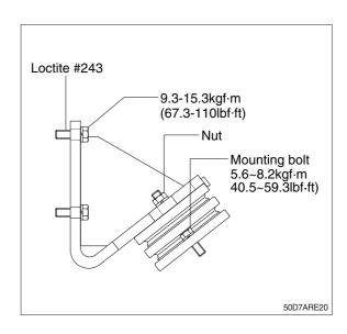
(3) Tightening torque of mounting bolt installing to torque converter housing.
